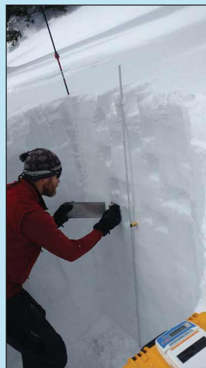
Density measurements being performed by Gus Goodbody. A 1000 cc sample of snow is extracted and weighed to calculate its water equivalent. Picture by HP Marshall. From SnowEx Winter Campaign 2017, Flickr site.
